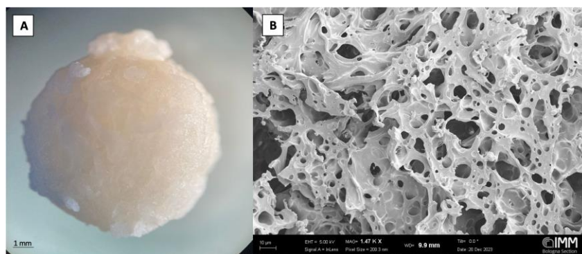
Figure 15. A) BSA-NPs sponge-like hydrogel, B) SEM image of a BSA-NPs sponge-like hydrogel freeze-dried.
